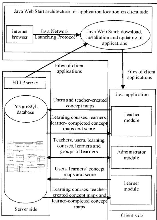
Fig. 5. The client/server architecture of the system.
